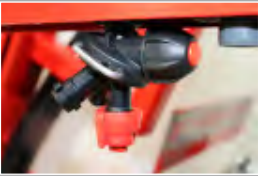
Triple nozzle holders fitted with red nozzles
