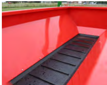
Cleated conveyor belt for effective sand delivery
