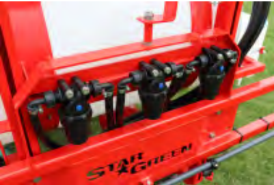
Triple filters for the spray booms
