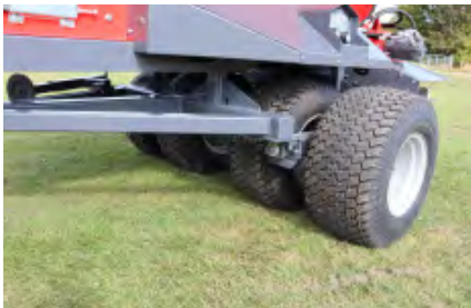
Pivoting axles spread the load on the turf tyres
