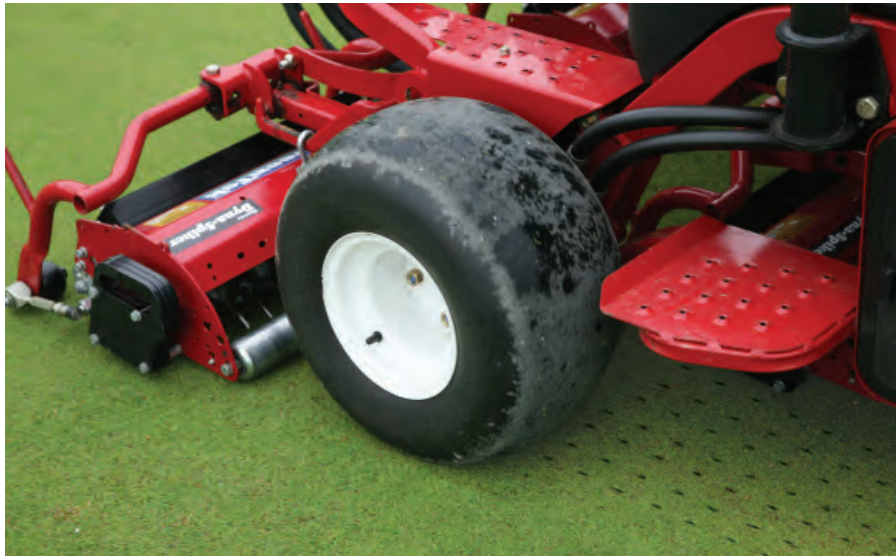
The Dyna-Spiker produces neat deep slits and an undisturbed surface
