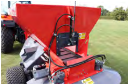
Hydraulic gate closes when belt stops to avoid loss of dry sand
