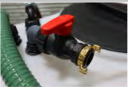
Mains water connection for tank rinsing
