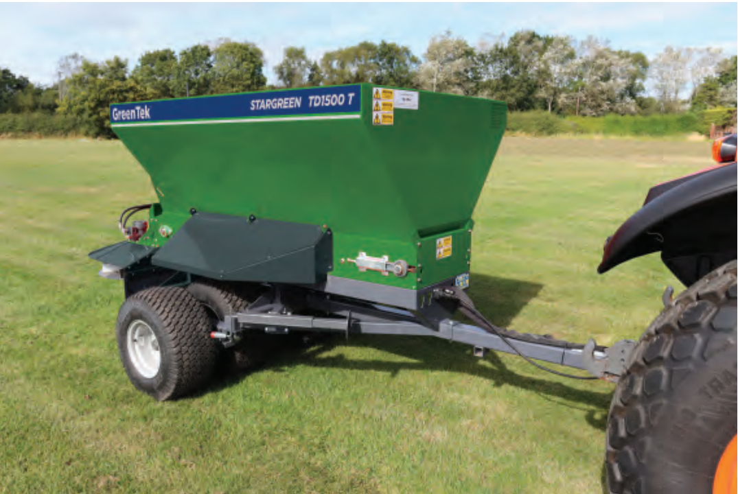
Large 1500l hopper holds 2.5 tonnes of sand
