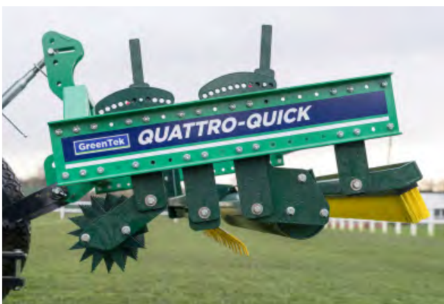
The Spring Rake is adjustable for intensity of grooming and thatch control
