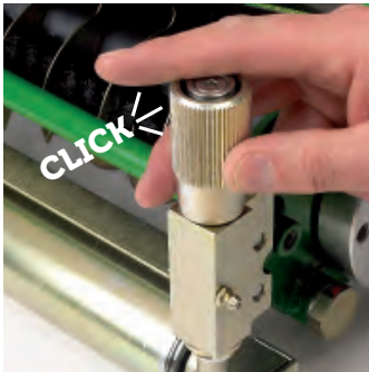
Each quarter turn click adjusts height by 0.25mm
