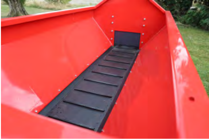
Smooth sided hopper has under-mounted sealing strips which avoid impairing the flow of sand onto the conveyor
