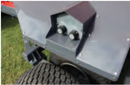
Belt and spinner speed adjusters with remote switching
