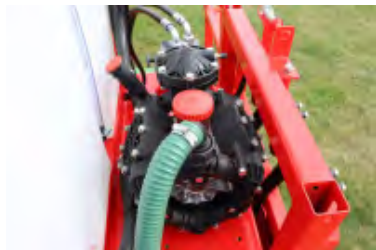
High-quality 3-cylinder diaphragm pump
