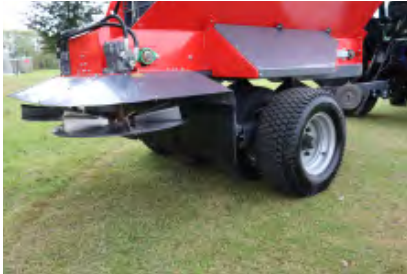
Twin hydraulic motors and stainless steel spinner discs
