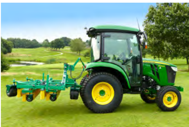
Hydraulically folded in for transport or topdressing
