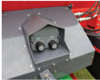
Speed controls with remote switching from cab
