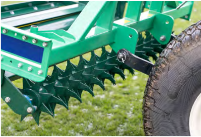
The Star Slitter aerates the surface to provide entry for air, water and nutrients
