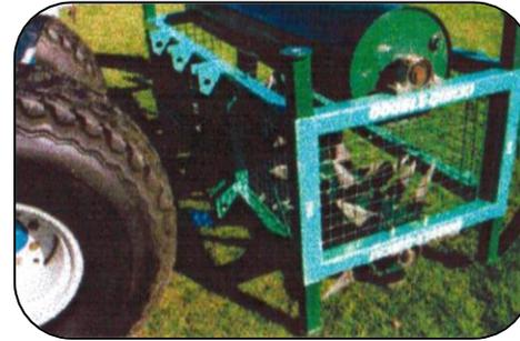
4. Uncouple the 3 point linkage and allow the frame to tilt over slightly onto the 2 rear stand legs.
