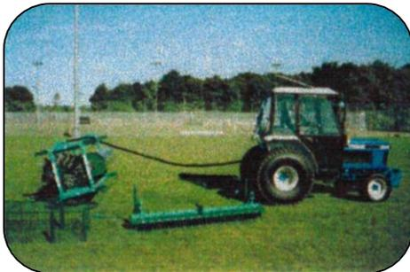
**9.** As soon as the Double-Quick starts to continue rolling under its own momentum STOP the tractor and allow it to come to rest on its 4 legs by itself.
