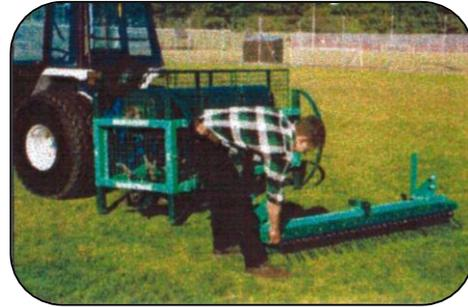
2. If a rear attachment is fitted, remove it by means of the 4 clevis pins and put it to one side.
