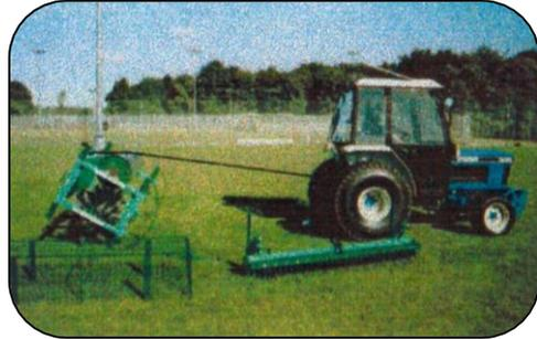
**8.** Ensure all bystanders keep back and drive the tractor very slowly forward causing the Double-Quick to rotate.
