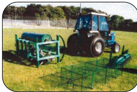
5. Drive the tractor round to the other side of the Double-Quick and reverse up to it squarely and centrally.
