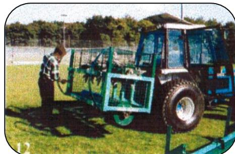
**12.** Raise the stand legs and lock up into the working position.
