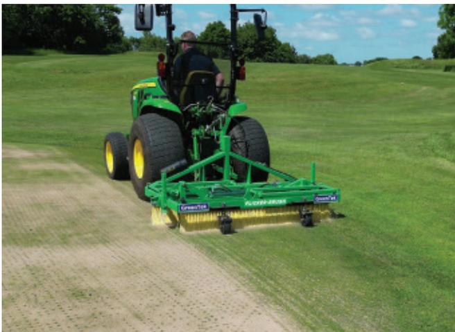
Hydraulically folds in to 2.2m for topdressing.
