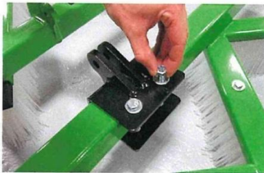
Attach extension wing brackets to the main frame of the Groomer. Do not tighten.
