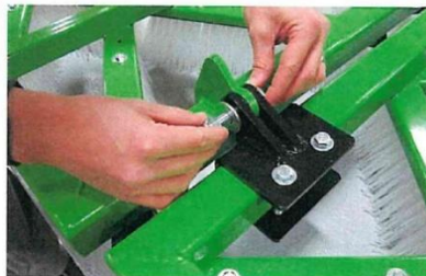
Attach each wing to the two extension wing brackets. Only tighten to a snug position so that the wings will fully rotate.
