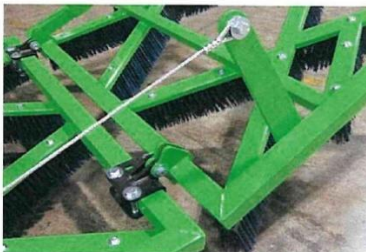
Attach the loose end of the cable to the upright arm of each wing.
