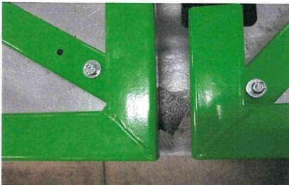
Align the frame of each wing with the frame of the Groomer. Fully tighten the two bolts of the extension wing brackets.
