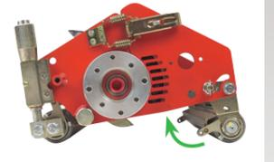
Two-position rear roller protects tungsten blade tips when storing and fitting the units
