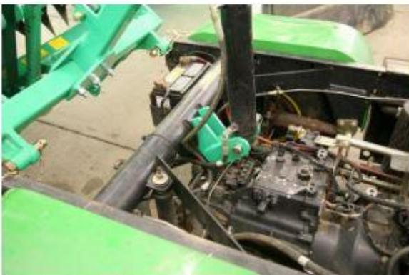
5. Refit hydraulic cylinder as shown.
