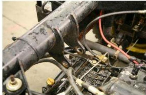
4. Rotate the hydraulic cylinder through 180°. Do not disconnect pipes.
