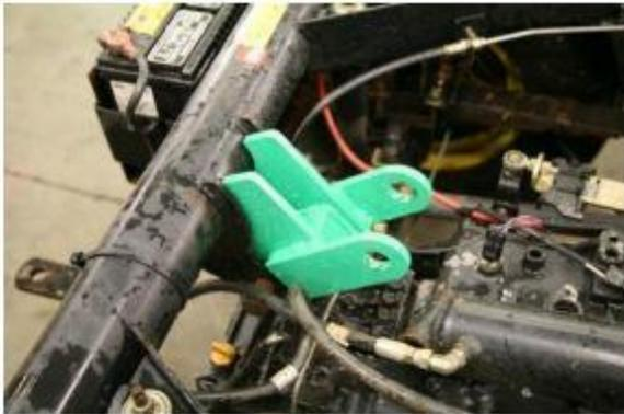
3. Fit the reverse cylinder bracket as shown.
