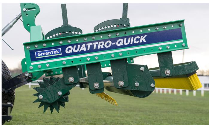
The Spring Rake is adjustable for intensity of grooming and thatch control
