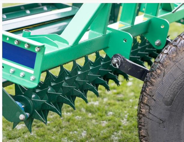
The Star Slitter aerates the surface to provide entry for air, water and nutrients
