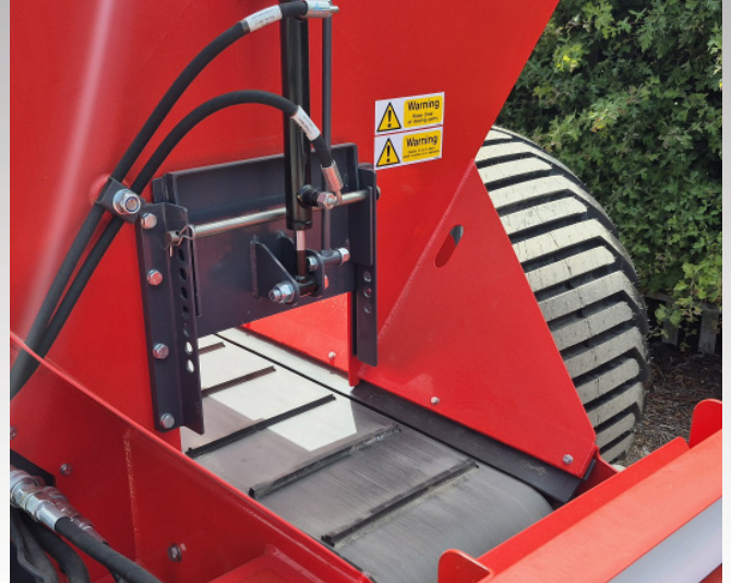
Smooth sided hopper has under-mounted sealing strips for unrestricted flow of sand onto the cleated conveyor
