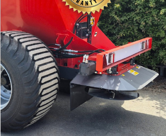
Twin hydraulic motors and 650mm spinner discs
