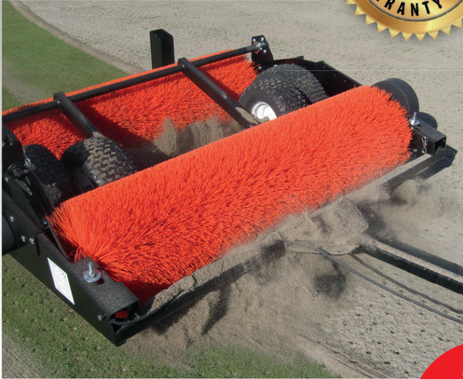
Sweep-N-Fill throws the sand upwards to fall straight down the holes
